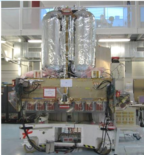
Service module with Li-ion batteries and plasma propulsion
