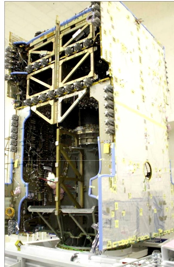
3-deck communications module
